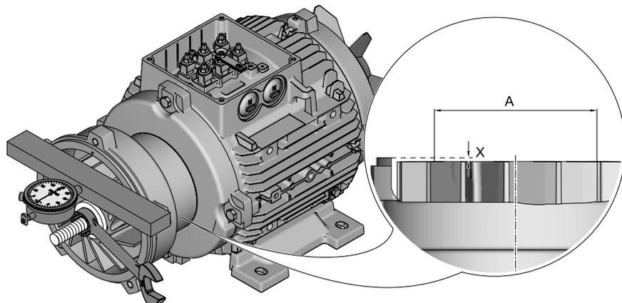
*Adjusting the clearance gap*
