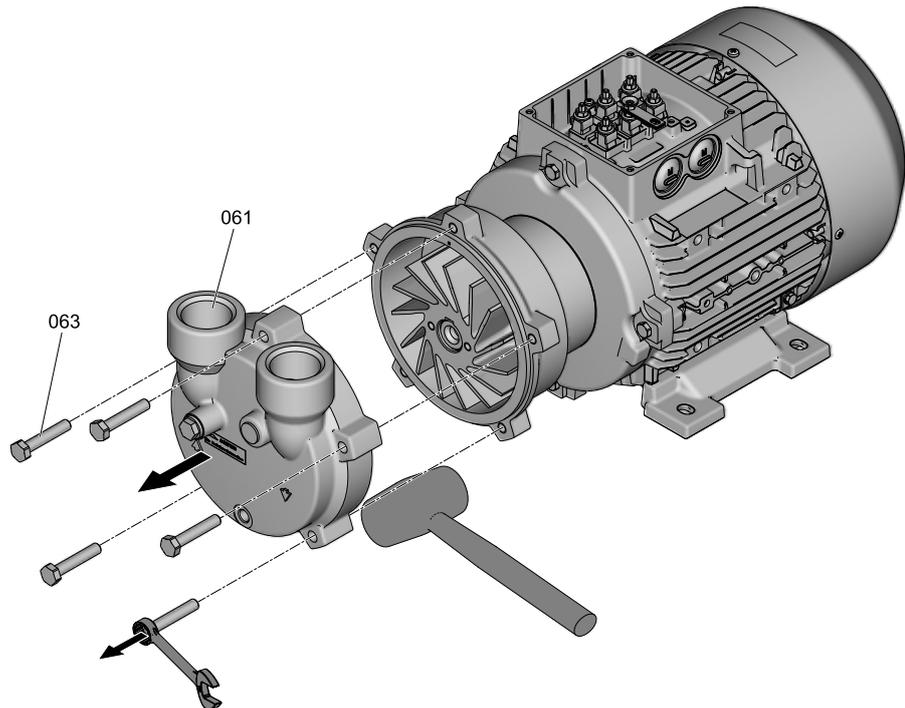
Removing the pump cover
