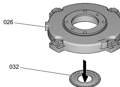
*Separating the sealing ring from the end plate*
