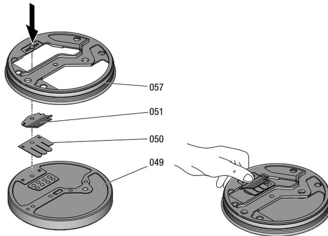
*Assembling the control disc*
