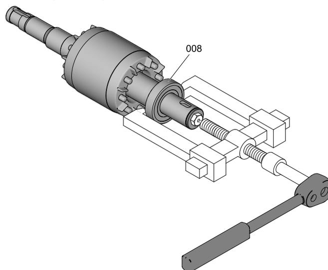
*Pulling off the motor side rolling bearing*
