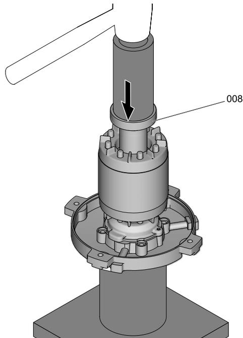
*Tightening the rolling bearing*
