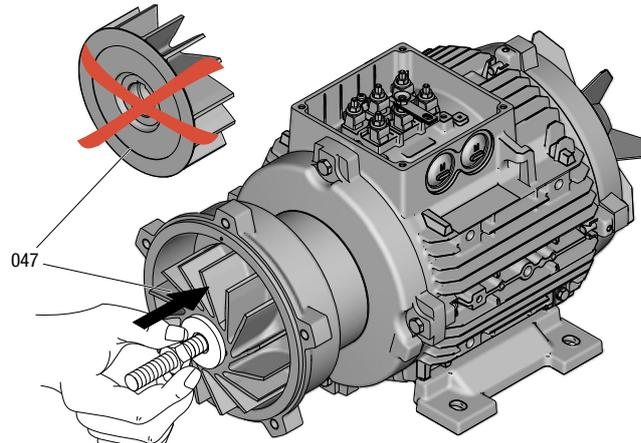
*Fitting the impeller*
