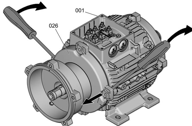
*Loosen the end plate on the pump side*
