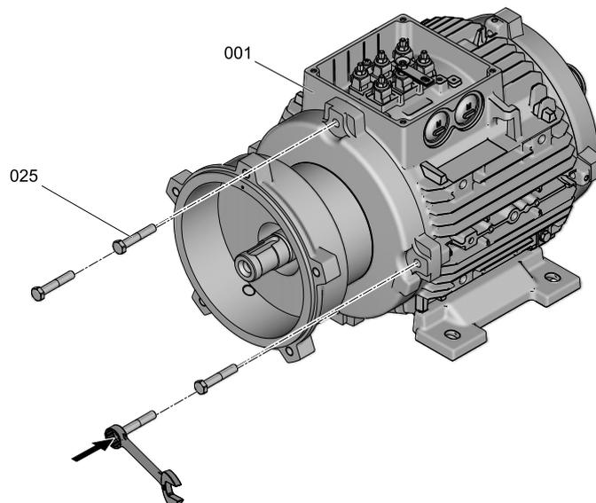
*Fitting the pump housing and motor housing*
