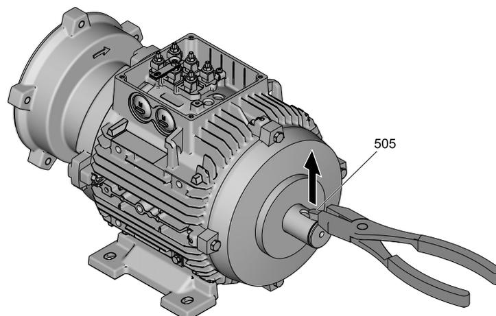
*Removing the exterior fan feather key*
