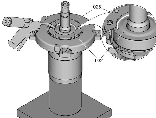
Sealing the end plate and the sealing ring
