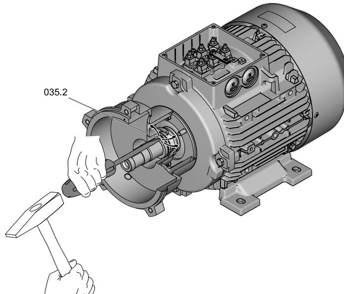
*Disassembling the counter ring from the rotary seal*
