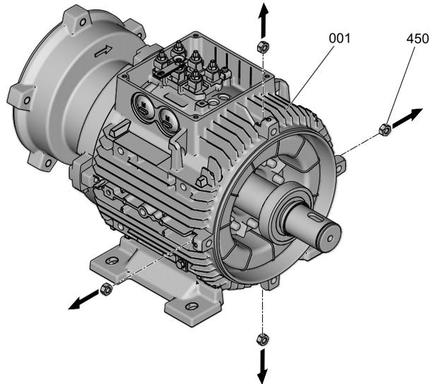
*Removing the nuts in the end plate on the ventilation side*
