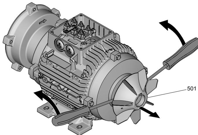
*Removing the exterior fan*
