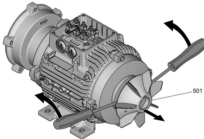
*Removing the exterior fan*
