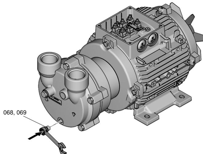
*Fitting the drain-off opening screw(s)*
