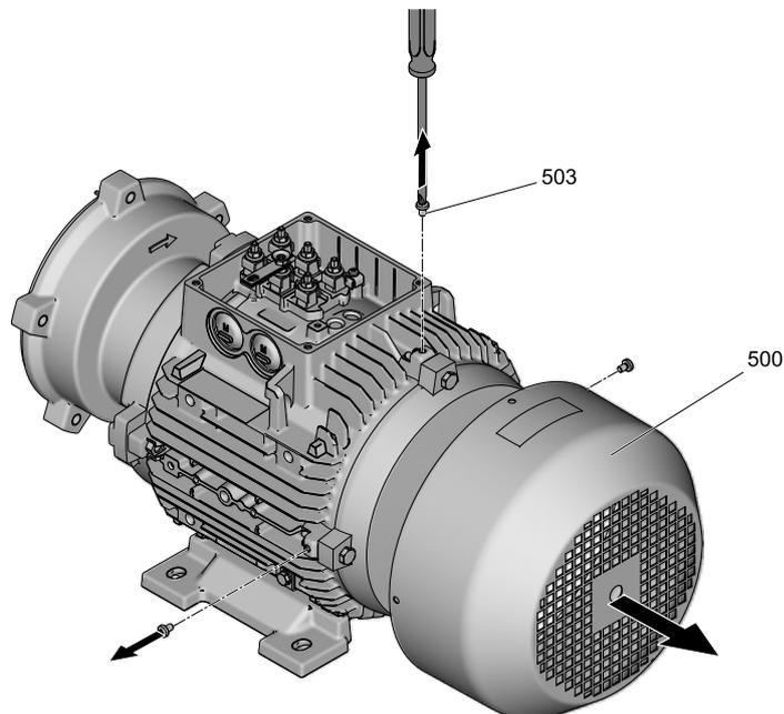
*Disassembling the fan guard*
