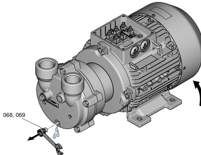
*Remove the drain-off opening screw*
