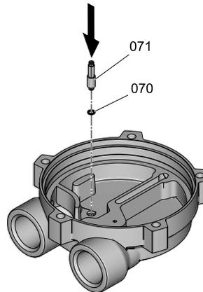
*Fitting the pipe for cavitation protection*
