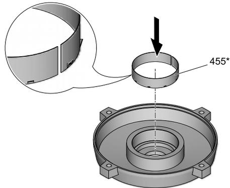
*Fitting the steel tape*
