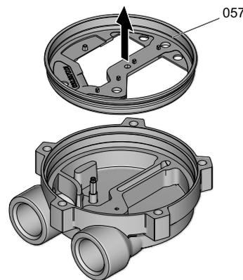
*Disassembling the seal of the control disc*
