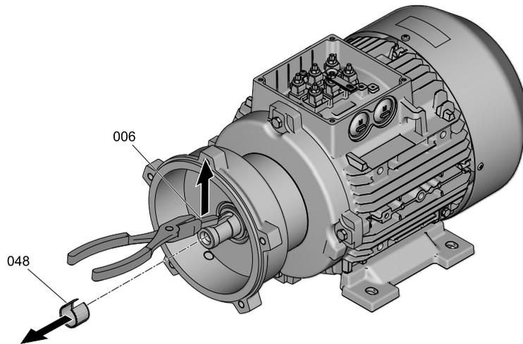
*Disassemble the feather key/tolerance ring of the impeller*
