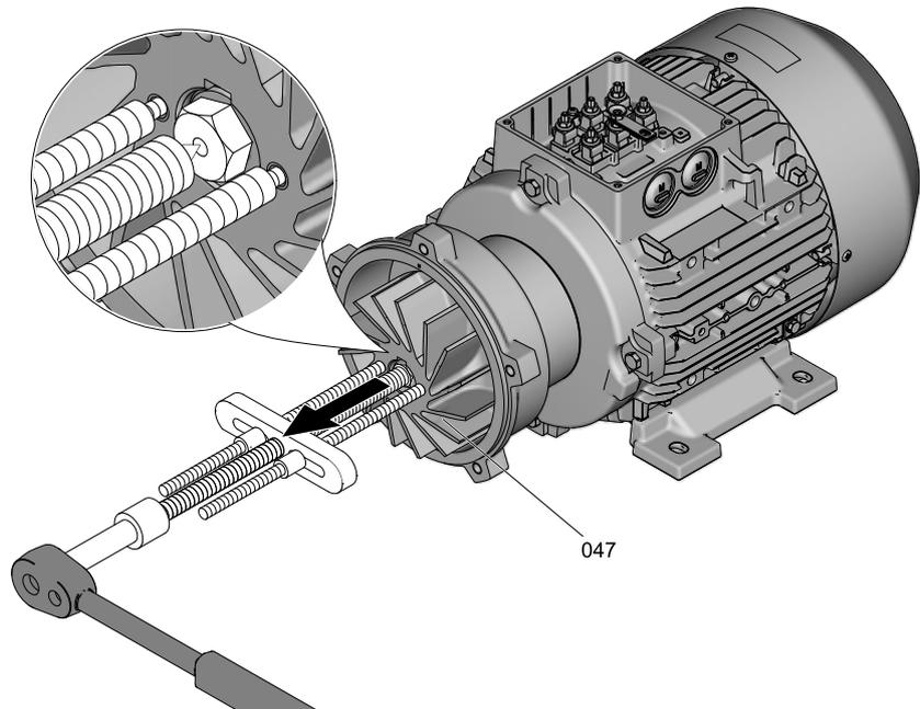
*Removing the impeller*
