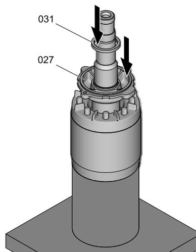
*Sliding the bearing cover onto the shaft*
