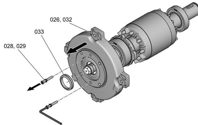
*Disassembling the end plate from the rotor*
