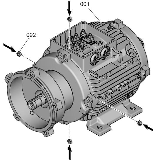
*Insert the pump side end plate nuts*
