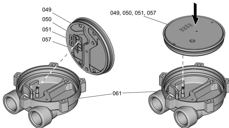
*Assembling the control disc and pump cover*
