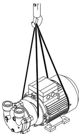
1. Run the lifting straps under the pump housing and under the fan cover and hook into the crane hook.
