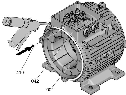
*Applying the sealant onto the motor housing*
