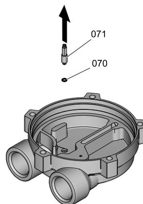
*Remove pipe for cavitation protection*
