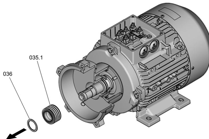
*Disassembling the rotary seal*
