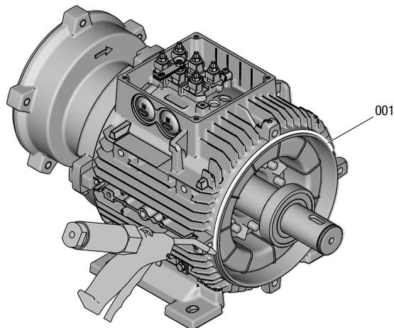
*Apply sealant to the ventilation side of the motor housing*
