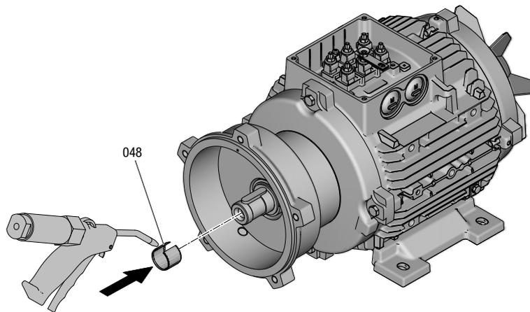
*Fitting the tolerance ring*
