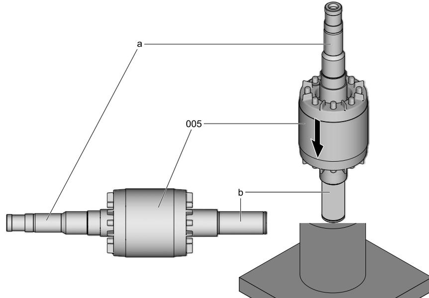
*Fitting the rotor into the assembly fixture*
