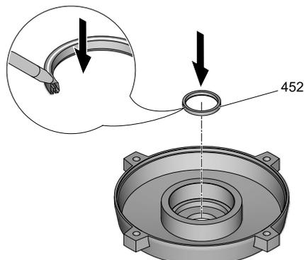
*Fitting the radial shaft seal*
