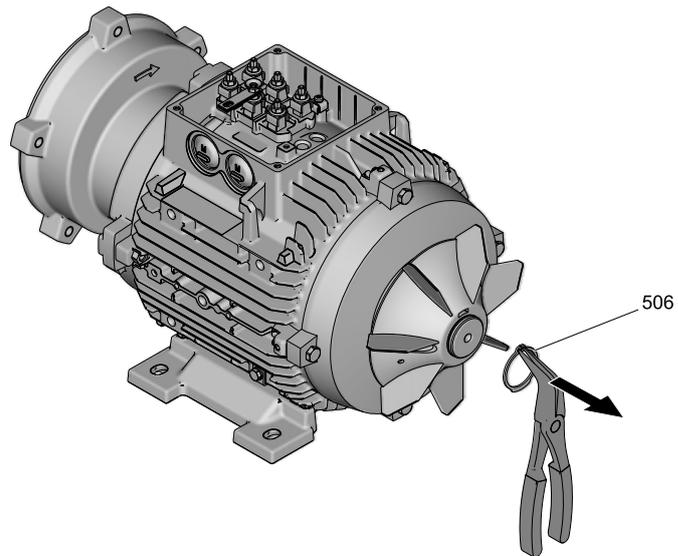
*Removing the exterior fan circlip*
