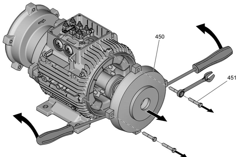
*Disassembling the ventilation side end plate*
