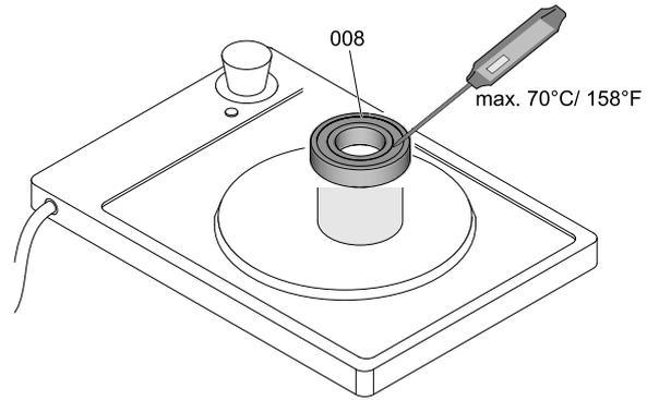
*Heating up the rolling bearing*
