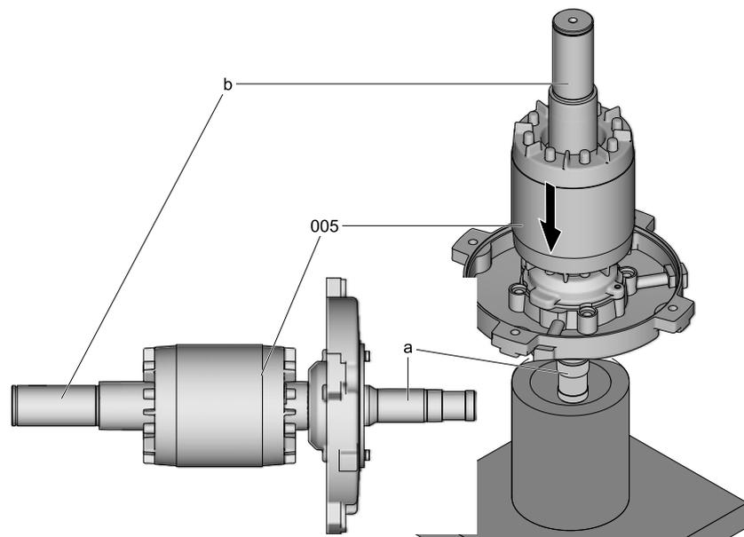
Fitting the rotor into the assembly fixture
