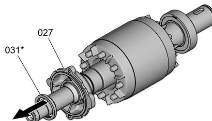
*Disassembling the bearing cover*
