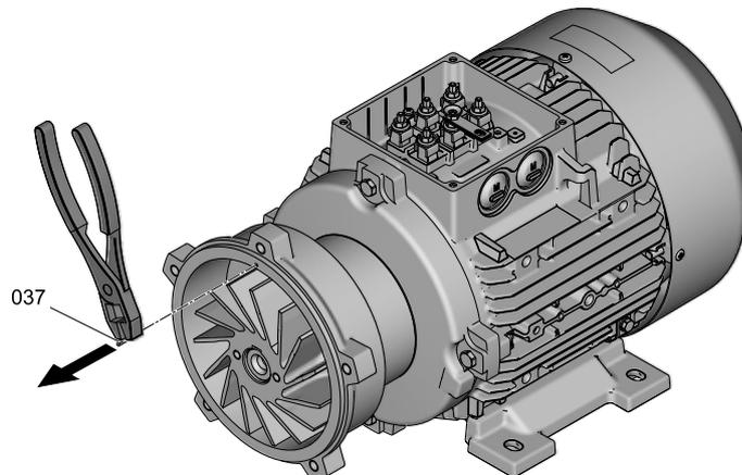
Disassembling the spiral locking pin
