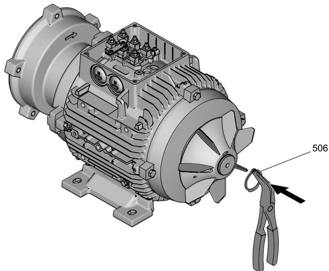
*Fitting the circlip of the fan impeller*
