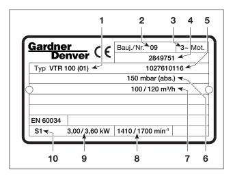
Fig. 5 Data plate (example)
