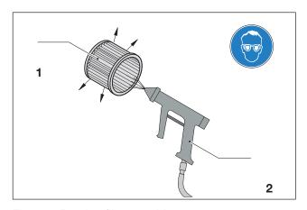
Fig. 8 Purging filter cartridge
