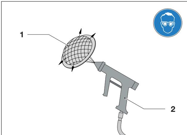
Fig. 5 Blowing out the mesh filter
